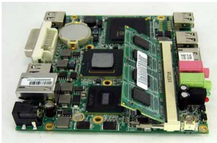
Place the RAM to the slot in push it down till the RAM is engaged.
