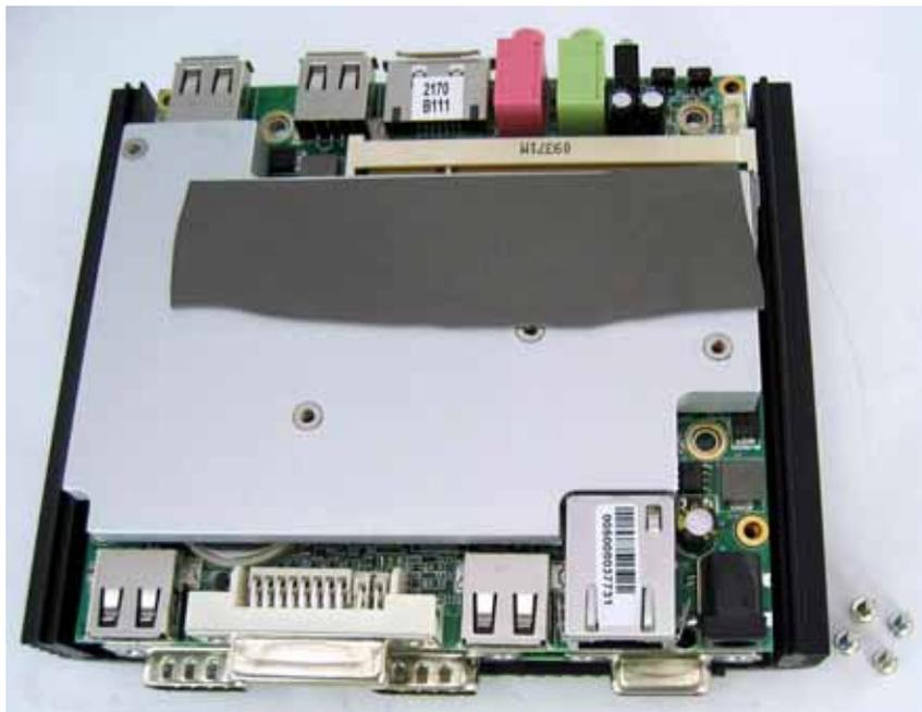
Hold the enclosure with one hand and remove the mainboard with you other hand upwards.
