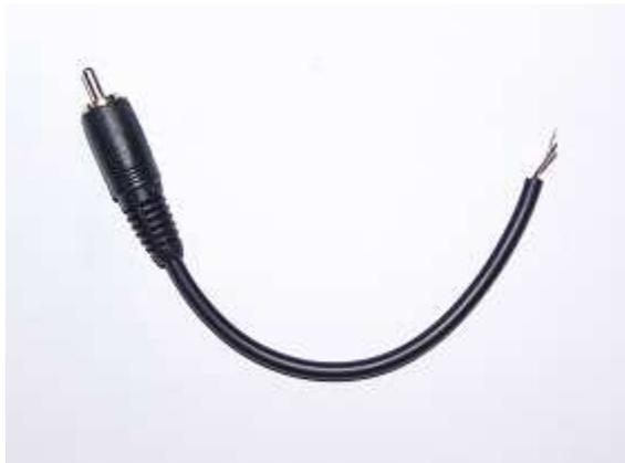
3. Attach shielding wire of RCA cable to white and green wire from white harness (soldering is the most reliable way to ensure tight connection)
