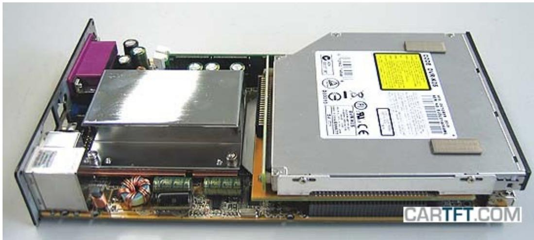
Before the motherboard gets slid in the case again, the fake-drive blend has to be removed of the case, so that the correct CD/DVD-ROM can be used.
